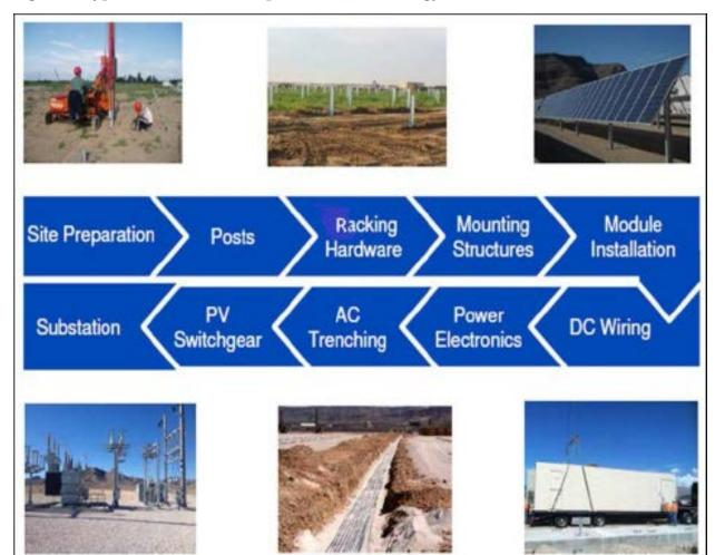
Figure 3: Typical Construction Sequence for Solar Energy Facilities
