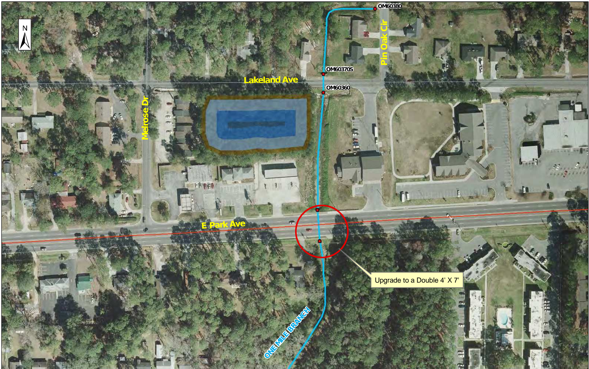
Figure 4.4.4 City of Valdosta, GA One Mile Branch Sub-basin Alternative OM2 Park Avenue Culvert Improvement and Regional Stormwater Facility near Lakeland Avenue
