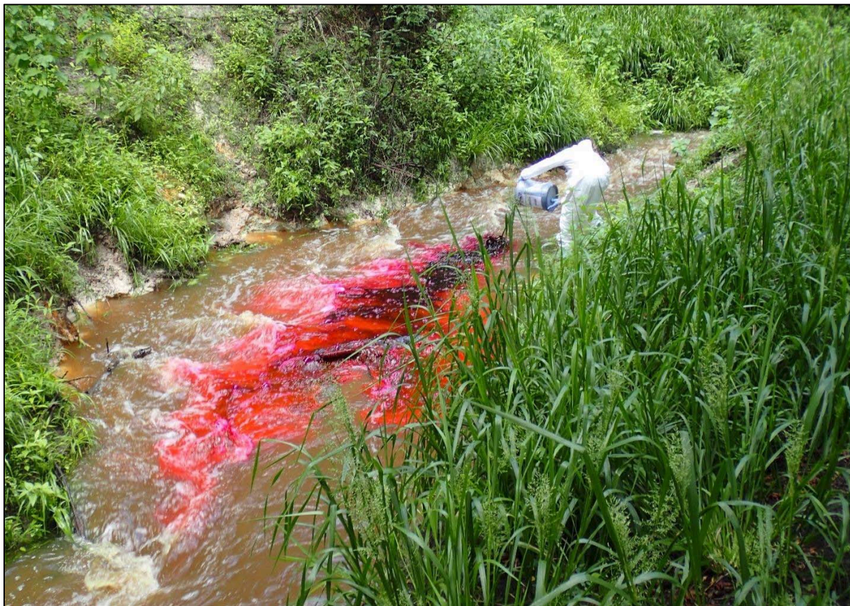
Figure 5. Dye introduction at Tiger Creek Swallet.
