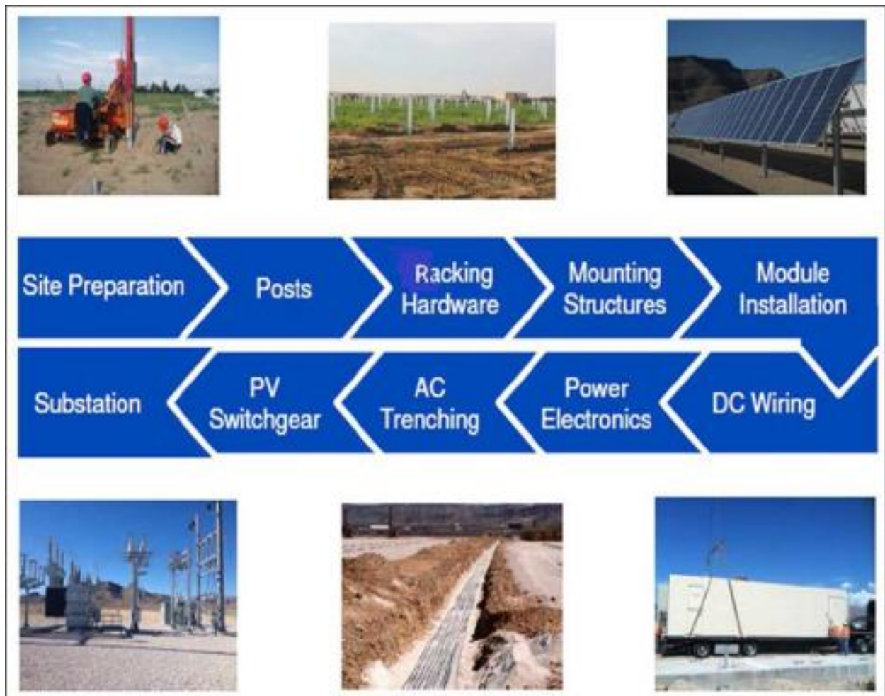
Figure 3: Typical Construction Sequence for Solar Energy Facilities
