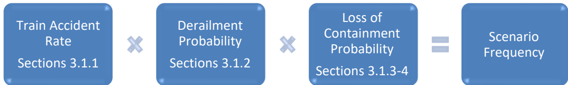
Figure 2. LNG DOT-113 train accident model overview.
