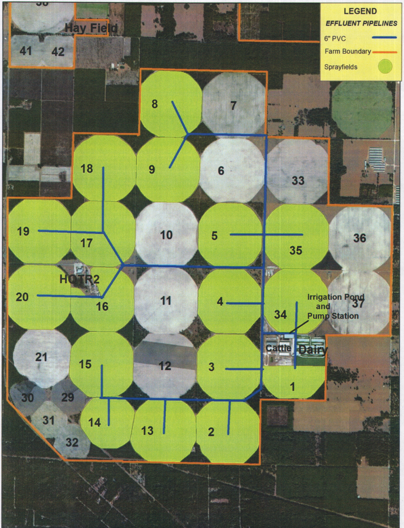
Figure 8. Sprayfields and Wastewater Effluent Pipeline.
