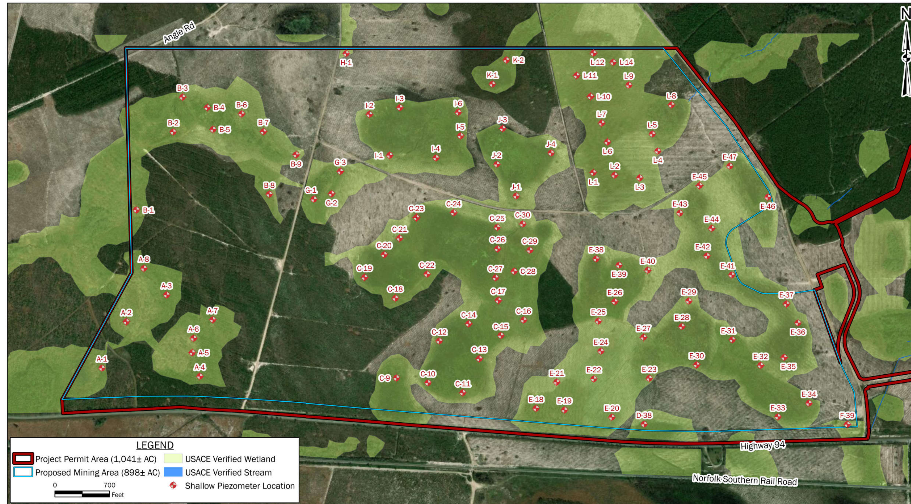
FIGURE 12: EXISTING SHALLOW "WETLANDS" PIEZOMETER LOCATION MAP TWIN PINES MINERALS ST. GEORGE, CHARLTON COUNTY, GEORGIA
