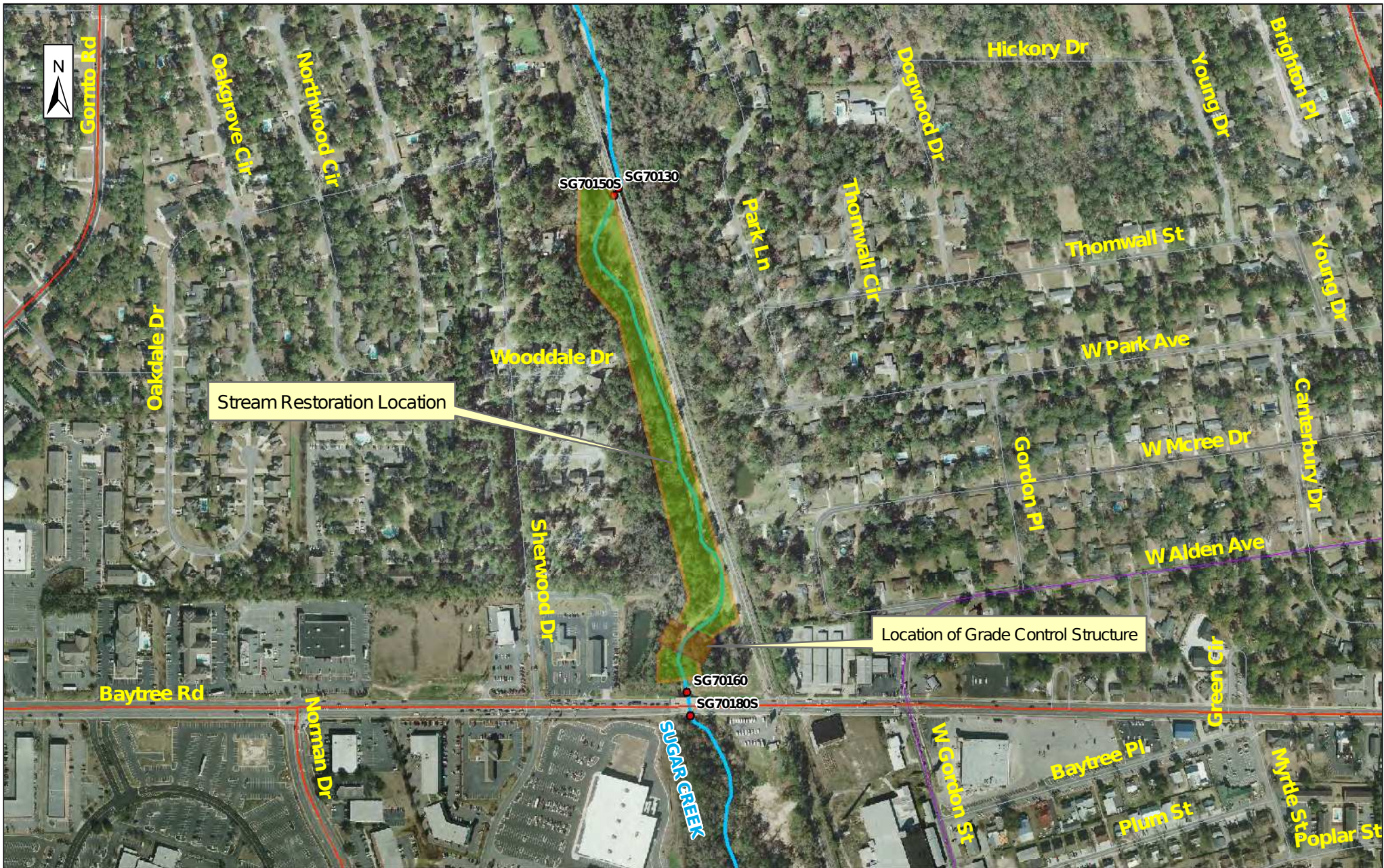
Figure 4.5.5 City of Valdosta, GA Sugar Creek Sub-Basin Alternative SG3 Sugar Creek Stream Restoration and a Grade Control Structure North of Baytree Rd
