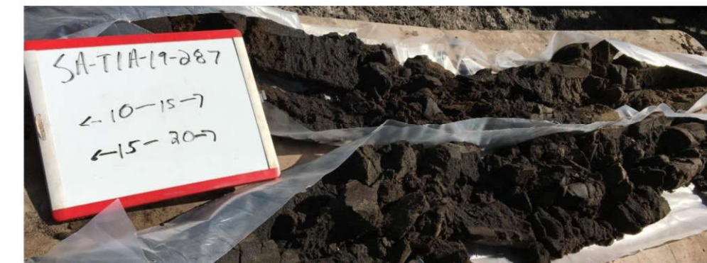
PHOTOGRAPH 3. UNCONSOLIDATED BLACK SAND
