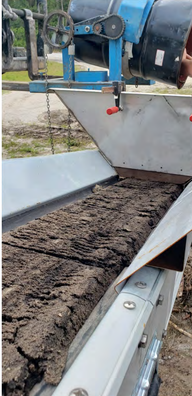
Photograph 3. Processing of UD drummed soil through mineral extraction processing plant by Mineral Technologies personnel.
