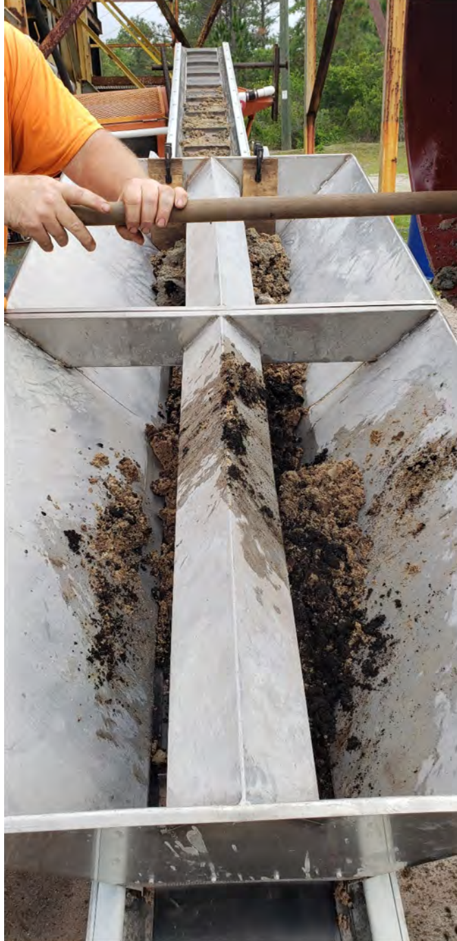
Photograph 2. Processing of UD drummed soil through mineral extraction processing plant by Mineral Technologies personnel.
