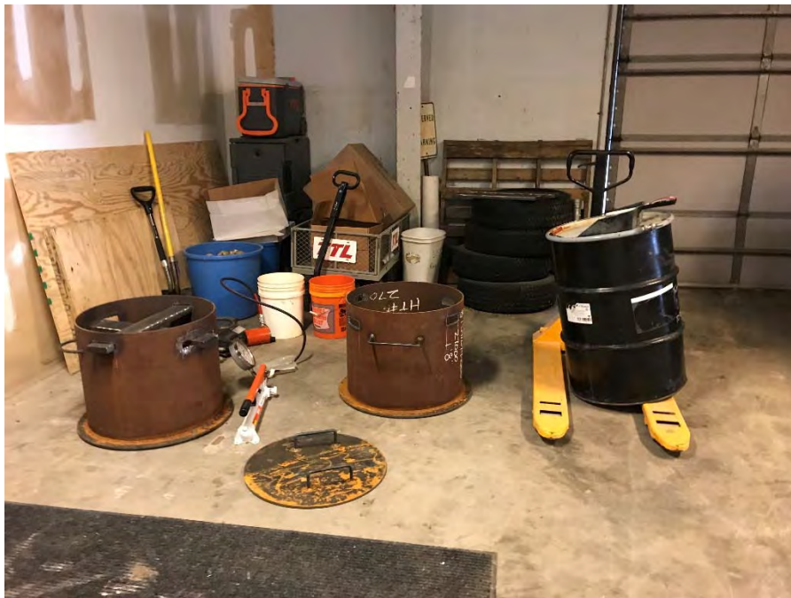
Photograph 9. Steel chamber used for applying load to processed sand.
