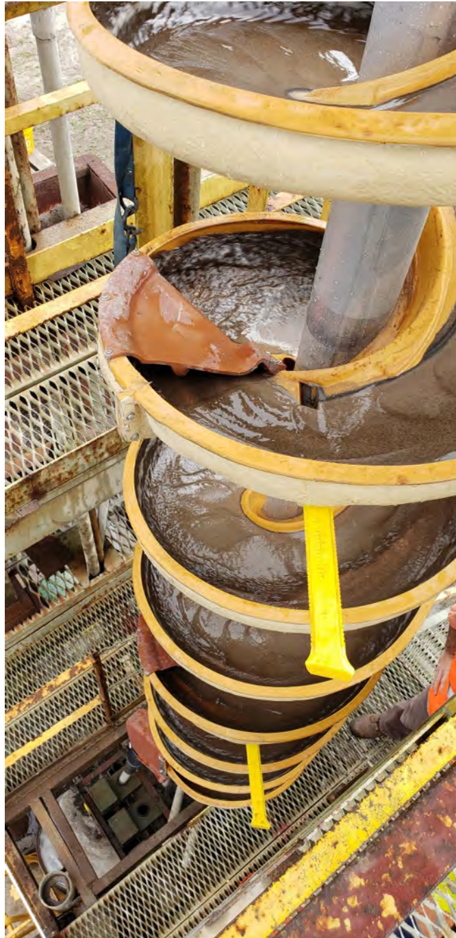
Photograph 5. Alternate view of sand mixed with water flowing through heavy mineral separation spirals.
