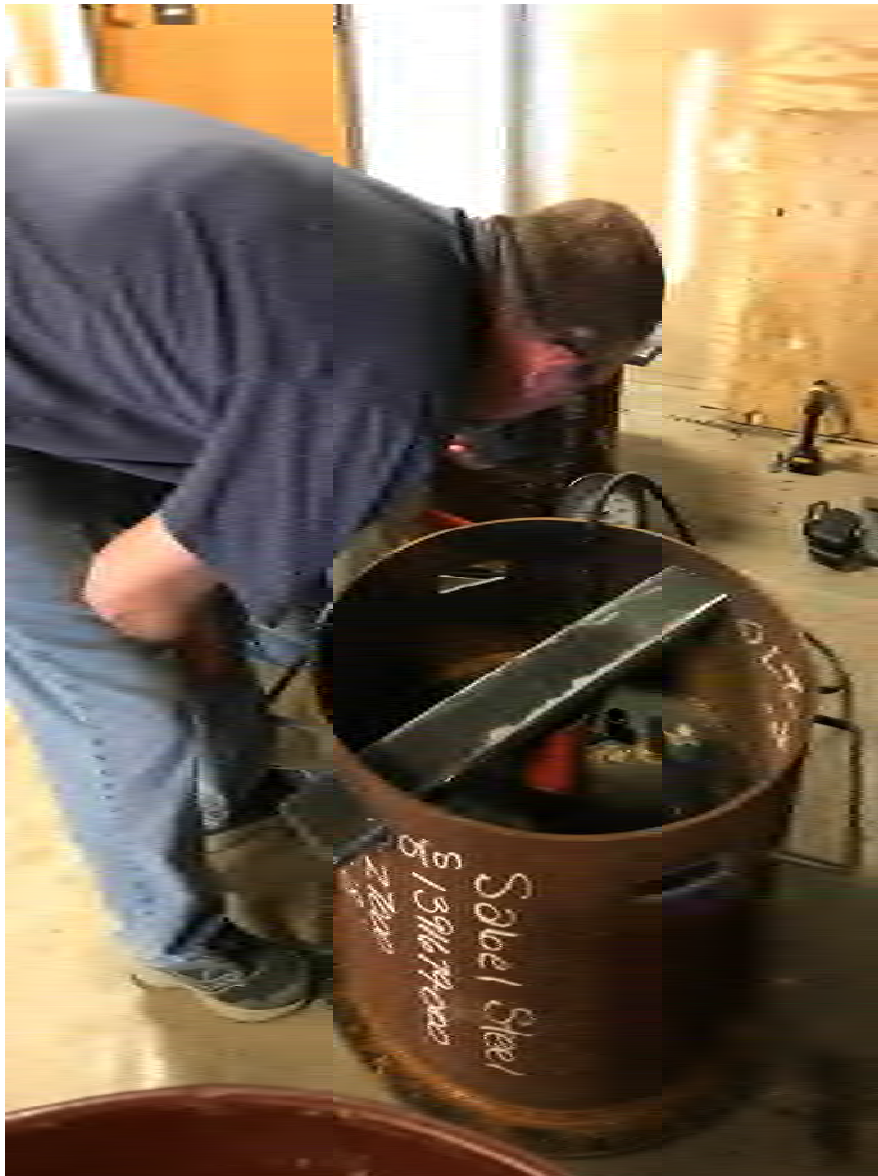
Photograph 11. Steel chamber sealed with lid for load application via pneumatic jack.
