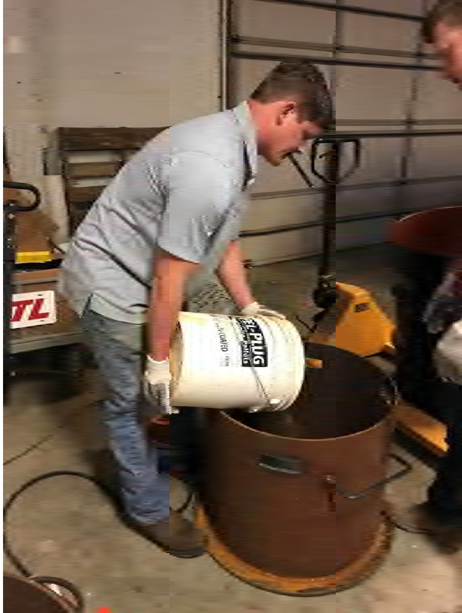
Photograph 10. Sand from drum UD338/25 being transferred into steel chamber.
