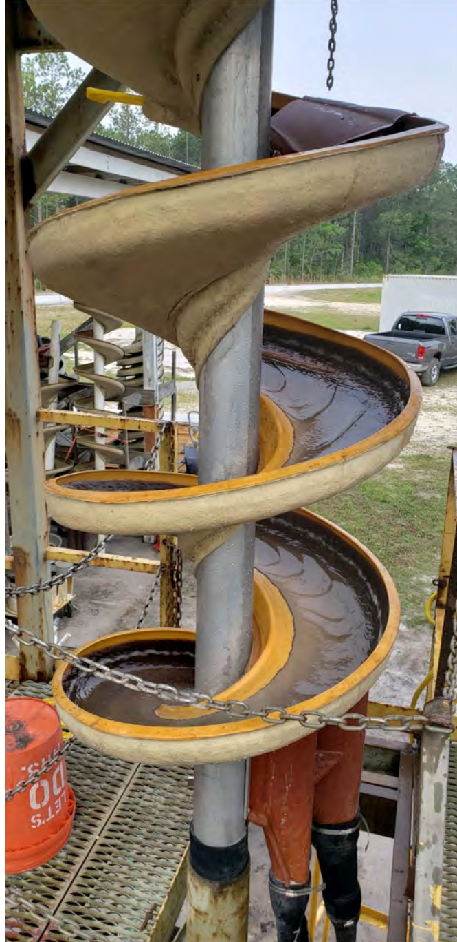
Photograph 4. Sand mixed with water flowing through heavy mineral separation spirals.
