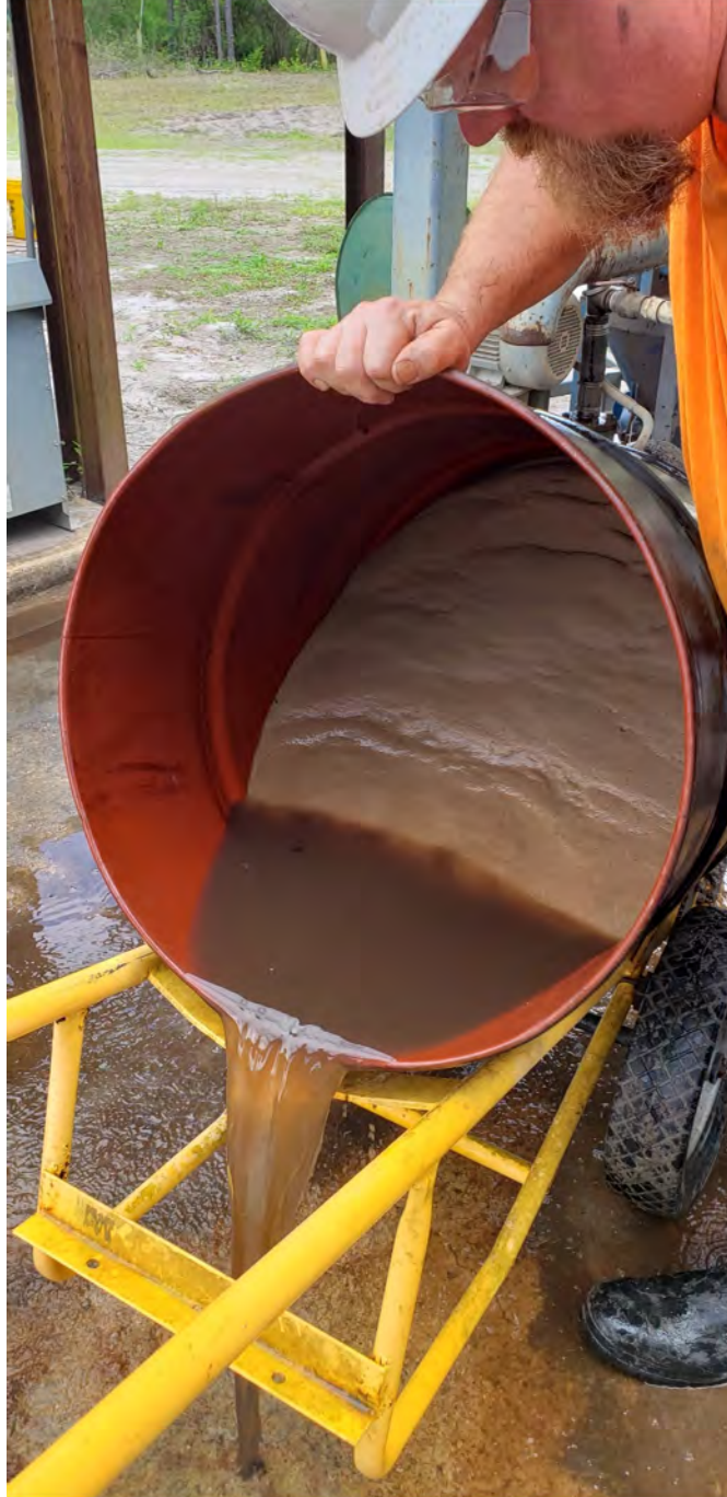
Photograph 7. Processed sand minus heavy mineral and any humate and/or clays returned to drum.
