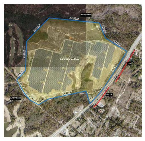
This project was built in 2015 including 143.39 acres for a 30 MW project with the closest home at 285 feet from the closest solar panel with an average distance of 719 feet.
