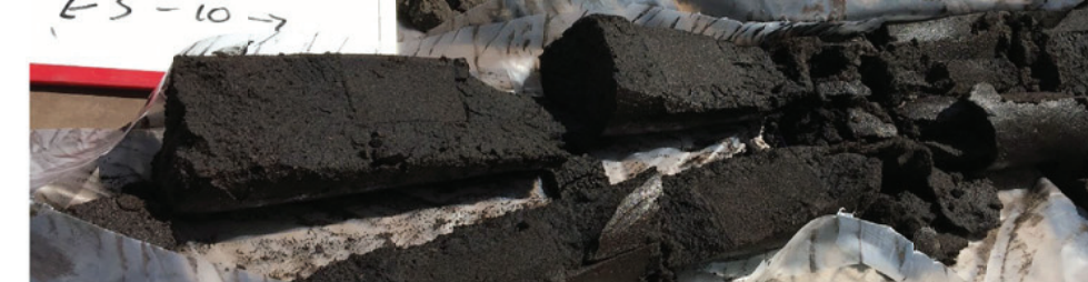
PHOTOGRAPH 2. SEMI-CONSOLIDATED BLACK SAND
