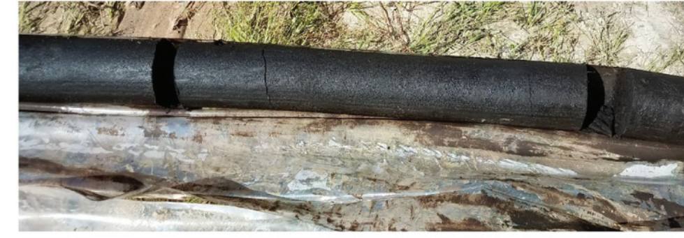
PHOTOGRAPH 1. LOW PERMEABILITY HUMATE-CEMENTED CONSOLIDATED BLACK SAND
