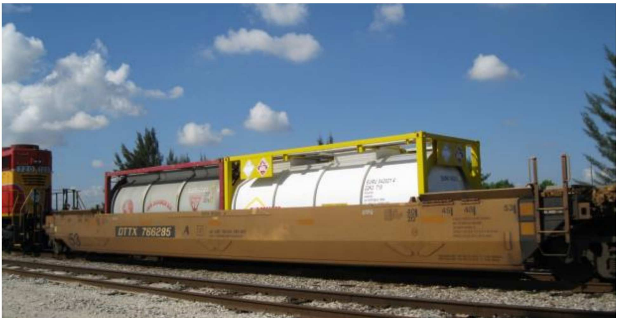
Figure 9. Representative well car in FECR intermodal yard containing two 20-ft ISO portable tank containers. One LNG ISO would replace these two containers in the proposed service.
