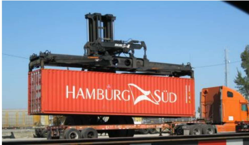
Figure 8. (b) (4) used for Lift On/Lift Off of intermodal containers.
