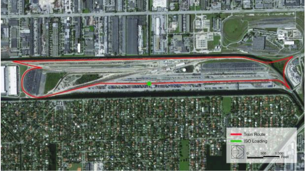
Figure 31. Aerial view of the Hialeah Yard. The train route along the outside yard rail lines is red and a representative location of lifting operations is shown as a green dot.
