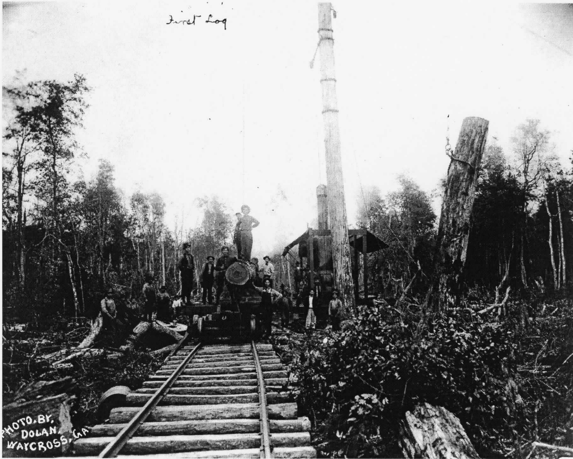
First Log, 1909. Overhead skidder cleans up about 28 acres from one spar or "head tree." Pulls in and loads logs at the same time (Photo by Dolan, Waycross, Georgia and in Hopkins, 45 Years with the Okefenokee Swamp , 1947).
