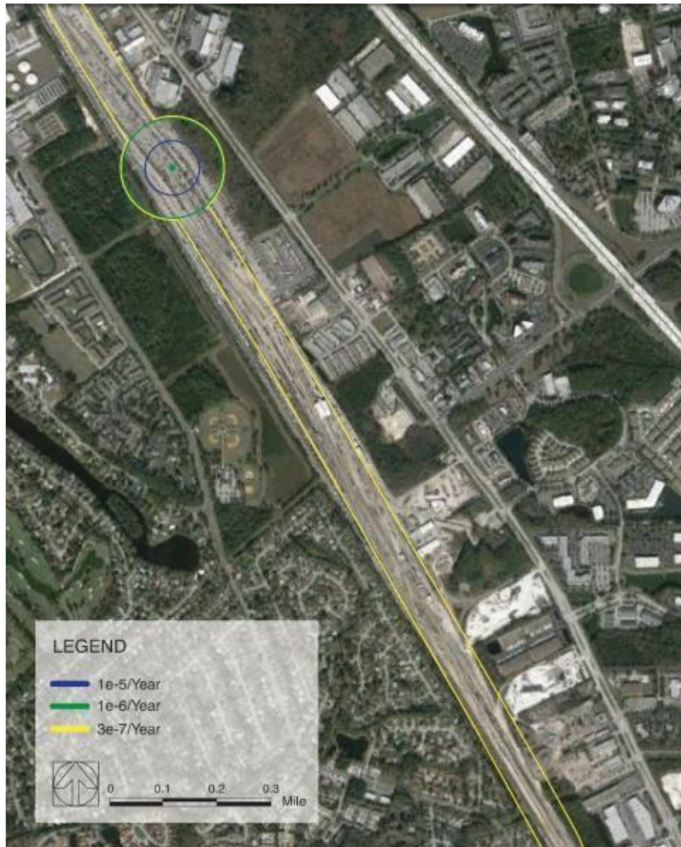
Figure 53. The cumulative IR contours for the Bowden Yard for baseline train configuration C-1. North is up.
