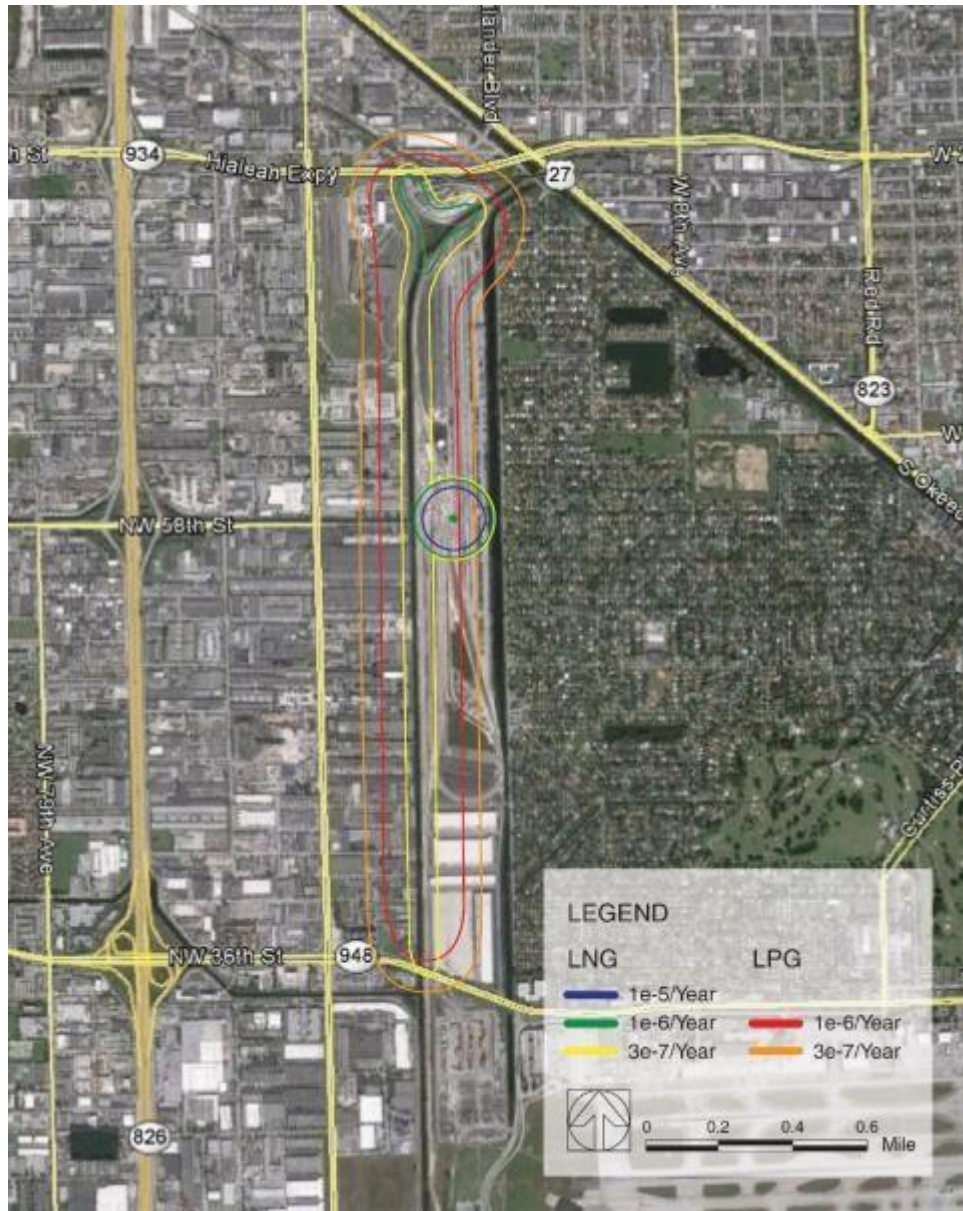
Figure 57. Comparison of IR contours for the movement of LNG ISOs and LPG in the Hialeah Yard.
