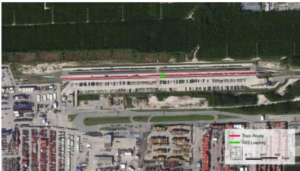
Figure 34. Aerial view of the Port Everglades intermodal facility. The yard rail line is red and the approximate location of lifting operations is represented as a green dot.
