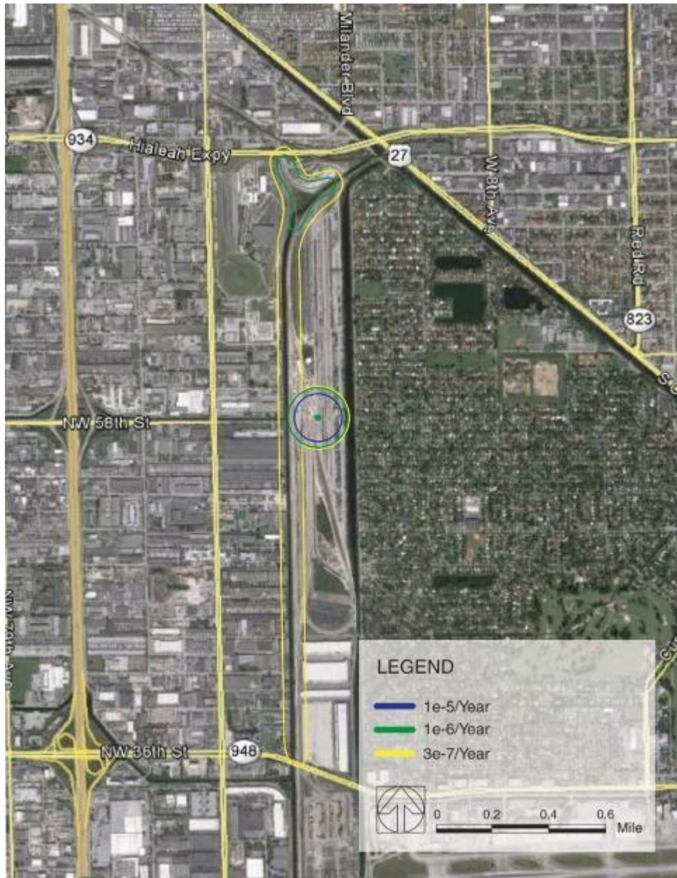
Figure 46. The IR contours for the Hialeah Yard and baseline train configuration C-1 using Route A.
