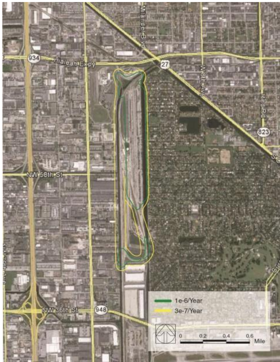
Figure 47. The IR contours for the Hialeah Yard and baseline train configuration C-1 using Route B.
