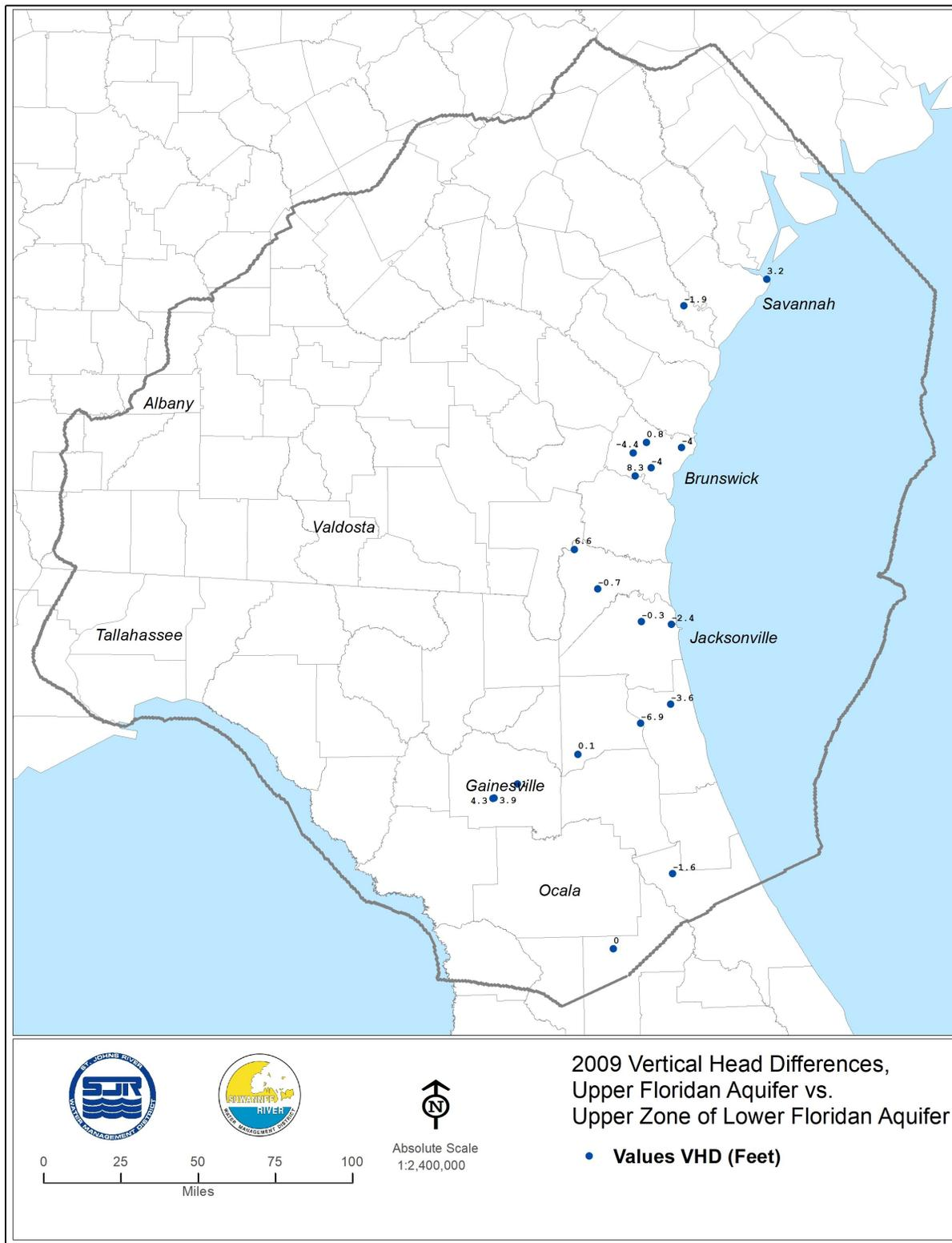
Figure 2-31. Middle confining unit vertical head difference, 2009 (Feet)
