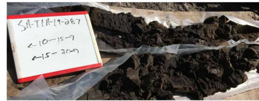
PHOTOGRAPH 3. UNCONSOLIDATED BLACK SAND
