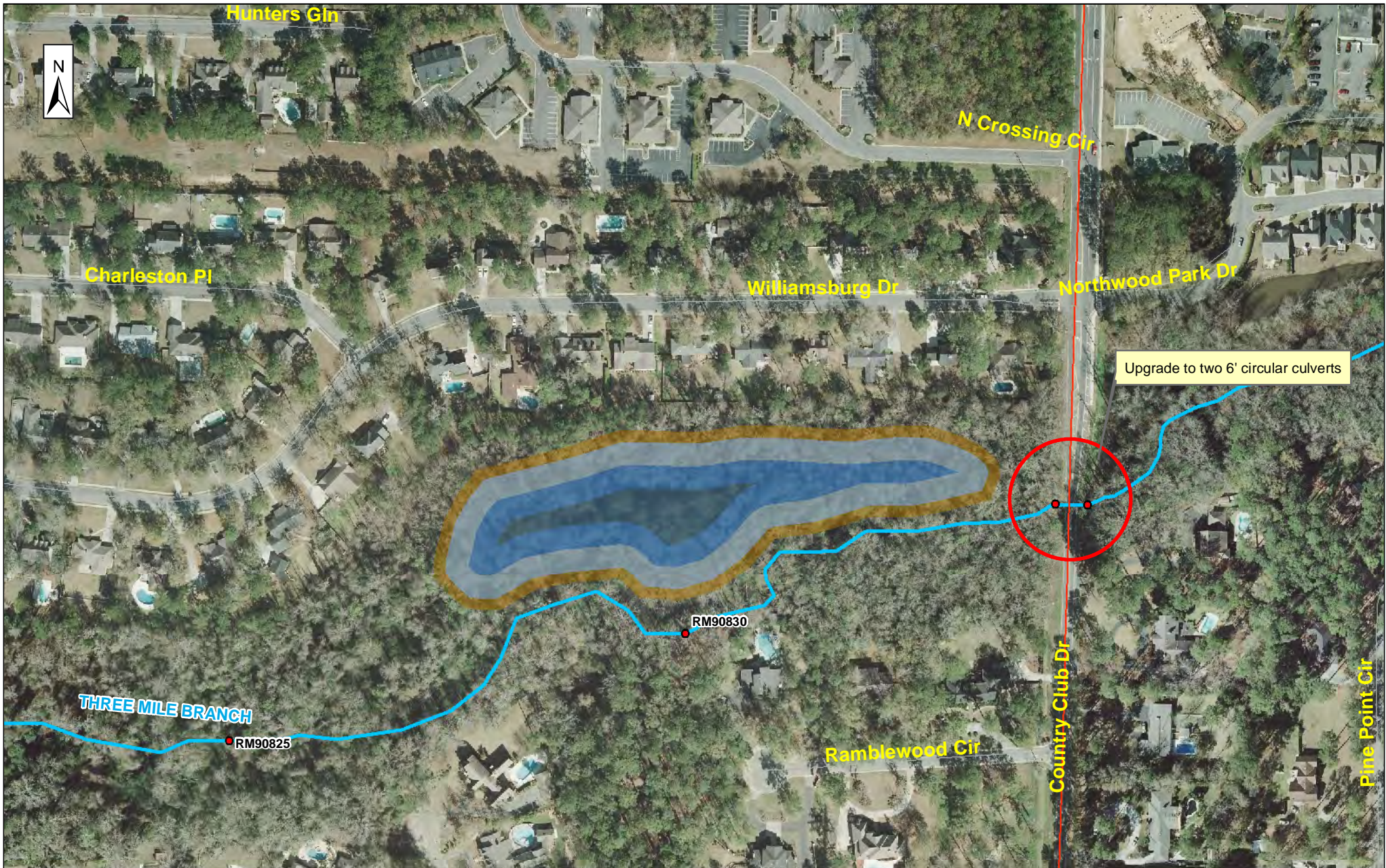
Figure 4.7.3 City of Valdosta, GA Three Mile Branch Sub-Basin Alternative RM1 Country Club Drive Culvert Improvement and Regional Stormwater Facility near Country Club Drive
