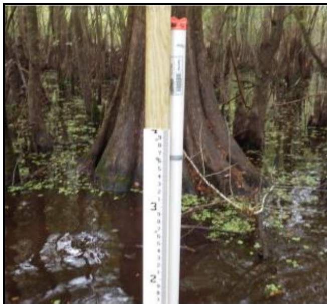
Figure 5B Typical Staff Gage Installation
