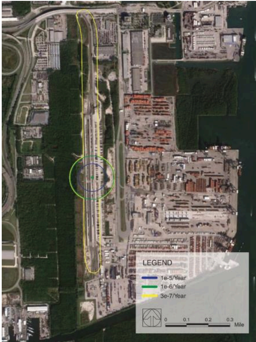
Figure 51. The IR contours for Port Everglades intermodal facility and baseline train configuration C-1. North is up.
