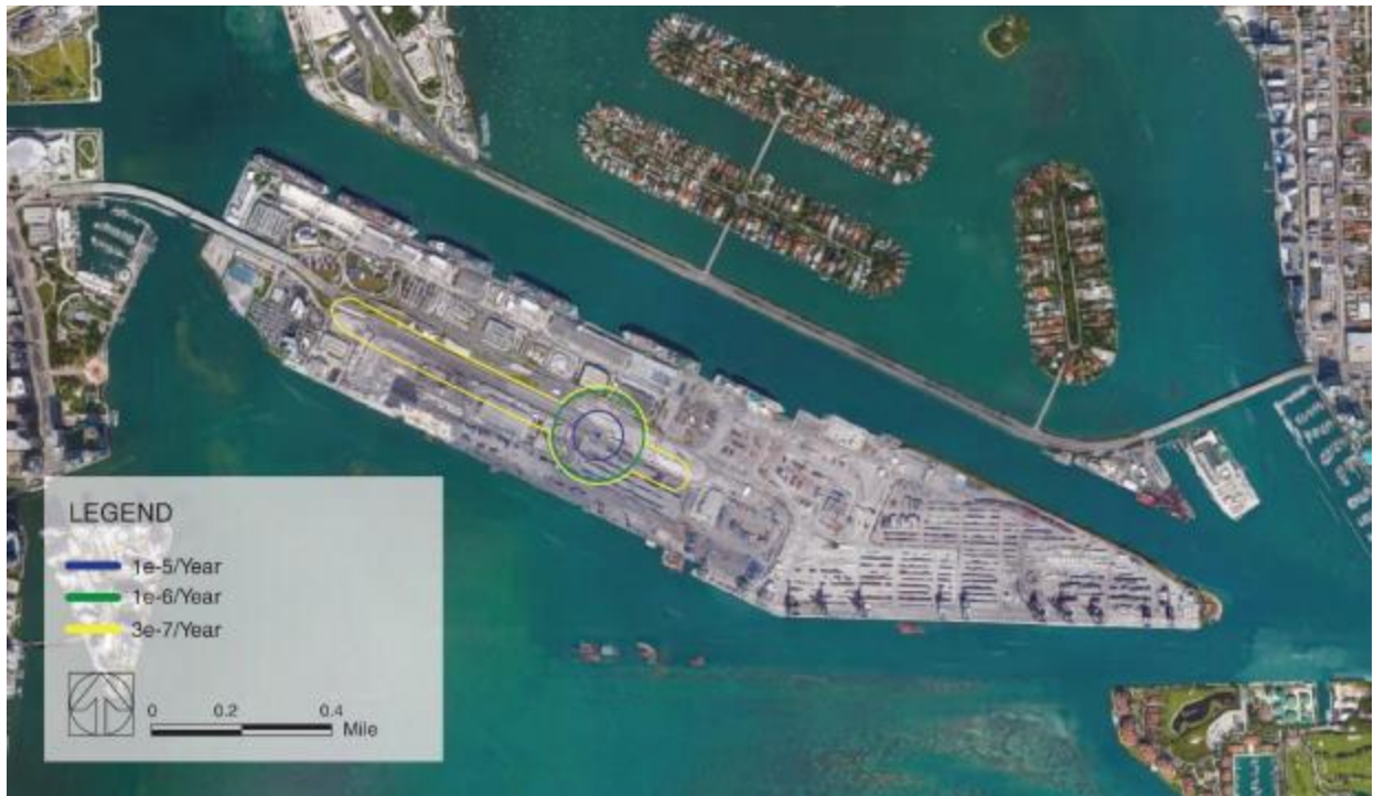
Figure 49. The IR contours for the Port of Miami intermodal facility and baseline train configuration C-1. North is up.
