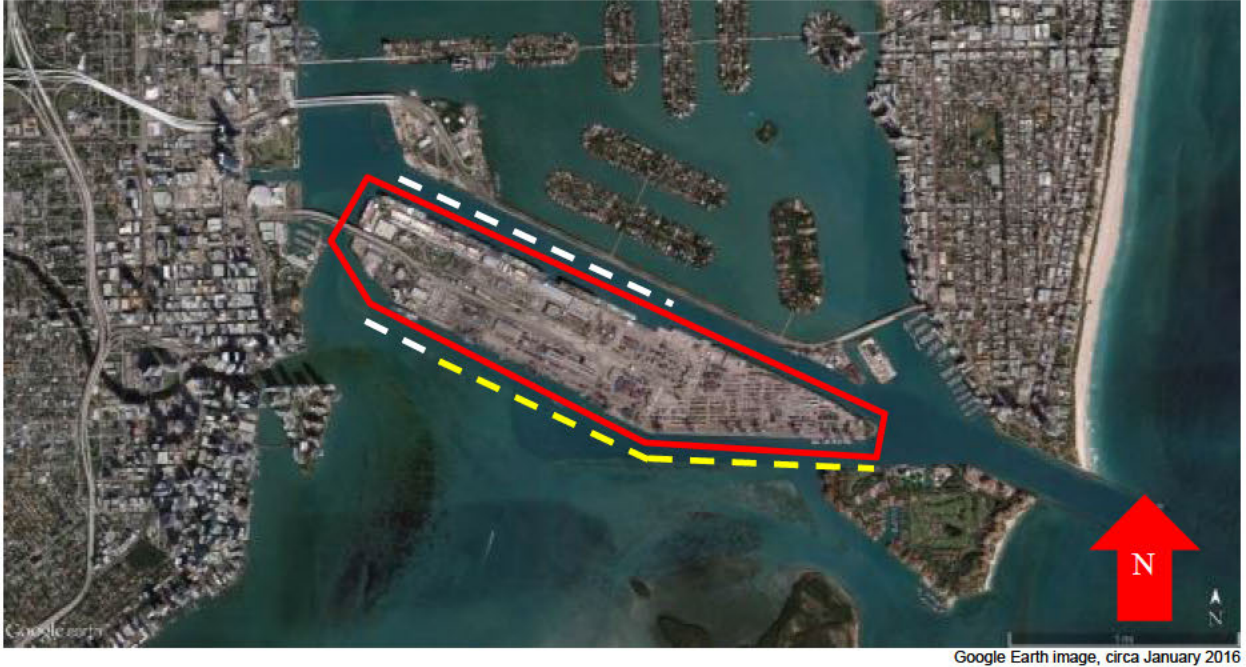
Figure 12. Dodge Island, which contains the Port of Miami (enclosed in red outline). The Port includes container ship docks (yellow hashed lines) and cruise ship docks (white hashed lines).
