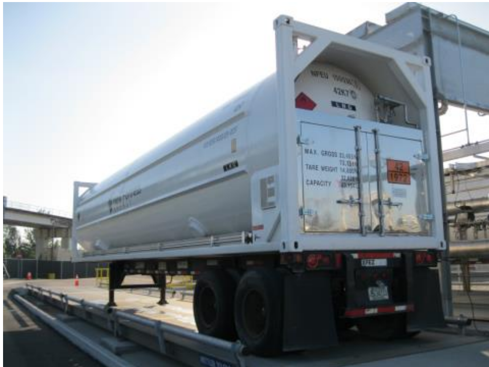
Figure 5. Rear view of (b) (4) ISO portable tank container on a truck chassis depicting the valve cabinet.
